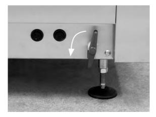
Fig. 6 Drain valve
