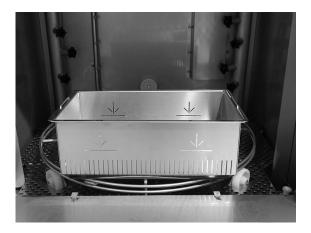
Fig. 30 Granule Collector in the machine
