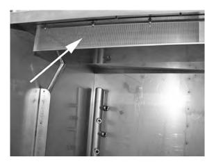
Fig. 41 EcoExchanger as seen inside the machine cabin
