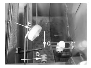
Fig. 36 Bottom sieve, level sensor and rollers
