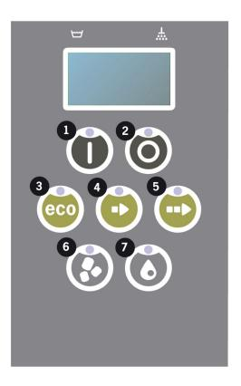
2 The Stop button is used to reset potential alarms.
