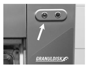
Fig. 21 When the program is finished the green light goes on.
