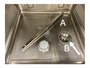
Fig. 14 Remove tank grid and filter
