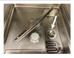
Fig. 17 Remove the filter
